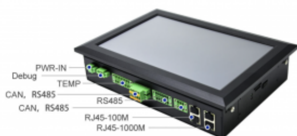
Connector Locations and Functions
