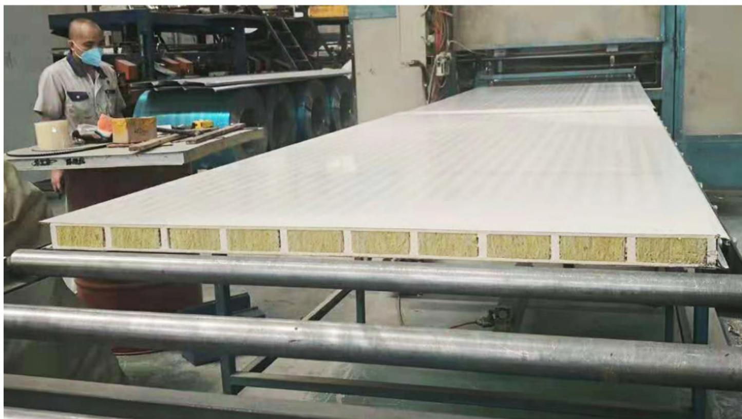
**Foshan, Guangdong Jan 12, 2026** ([Issuewire.com](http://Issuewire.com)) - The global demand for high-performance, fire-safe building materials has made the Magnesium Oxide (MGO) Rock Wool Sandwich Panel a product of critical importance. Combining the fire resistance of rock wool with the non-combustible and moisture-resistant properties of an MGO facing sheet, this panel represents the pinnacle of modern construction safety.
