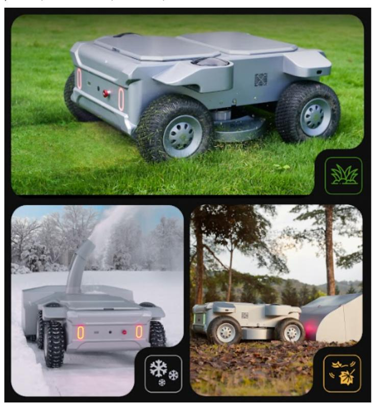
Management Robot is officially announced. Combining AI visual navigation, RTK precision positioning, and a modular operation system, this product provides comprehensive solutions for lawn care, snow removal, and multi-scenario yard management. Thanks to its modular design, users can effortlessly switch between multiple operation modes — such as mowing, snow blowing, leaf collection, loading, and towing — achieving versatile functionality. Apollo Turfstorm will be coming soon on Kickstarter.
