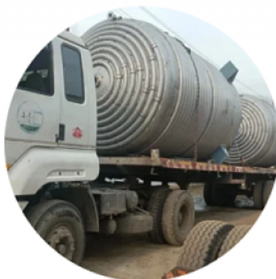
Limpet coil Reactor
