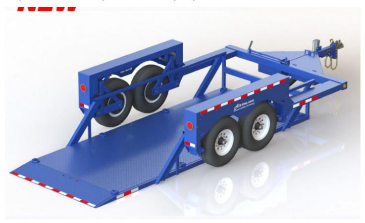
California, La Verne, Feb 11, 2021 (Issuewire.com) - Air-tow Trailers, the manufacturer that revolutionized the trailer industry with ground-loading technology, now offers models with 14,000-pound capacities. Every model in the Air-tow line lowers flat to the ground for simple and safe loading of all types of equipment. Air-tow Trailers make it easy to load with a pallet jack or transport heavy equipment without hassle.
