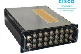
The Ethernet switch is offered in different standard configurations with support upto 24-ports Ethernet Connectors, Up to 4-Optical GigE Connectors. Layer 2 and Layer 3 switching, and routing is available to divide large networks into different subnets and allow data & information to communicate across the network. This switch comes with & without PoE support.
