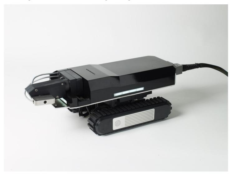
**Essex, Sep 5, 2019 (Issuewire.com)** - The new <u>robotic technology</u>, developed as a result of an extensive research and development programme, is the first of its kind in the industry. A defining feature is the system's ability to record videos and images of blockages, concerns and the cleaning taking place while automatically adjusting to warped tubes.
